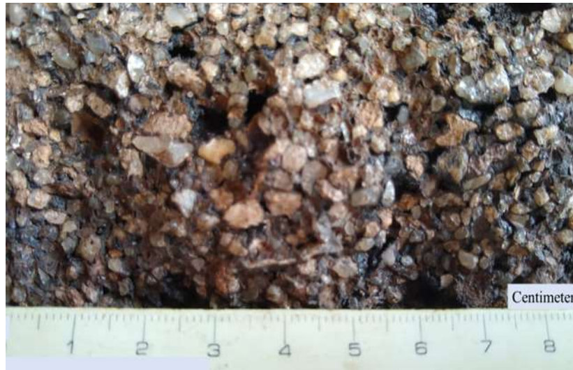
Figure 4. Detail of the structure of the laterite in the “Maracujá Deposit” (point 19 in Figure 1), showing the proportionality between the quartz-rich matrix and the ferruginous cement. The cement has the following chemical composition determined by X-Ray fluorescence: % \text{Al}_2\text{O}_3 - 2.4, % \text{SiO}_2 - 8.0, % \text{P}_2\text{O}_5 - 1.6, % \text{Fe}_2\text{O}_3 - 76.5, % \text{CaO} - 0.10, % PPC – 11.1.
