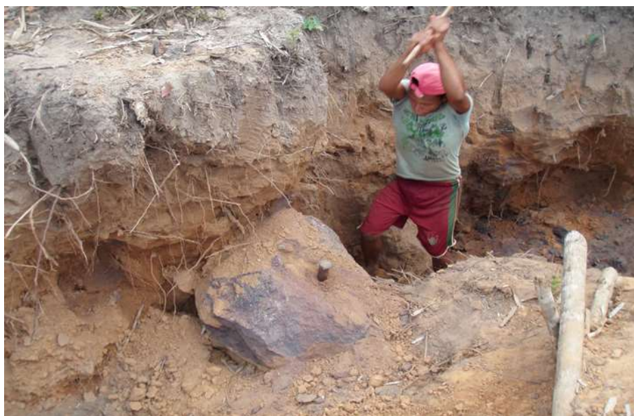
Figure 2. Lateritic coverage with variable thickness of 0.50 to 1.50 m. The image belongs to deposit/point 19.
