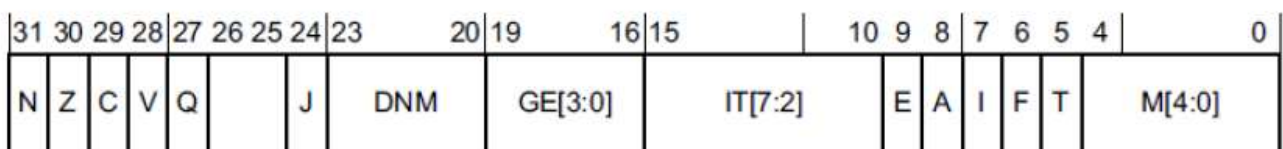
Figura 21 – Current Program Status Register no Cortex-R4. Fonte: ARM, 2009b.
