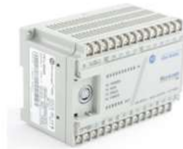
(c) Allen Bradley Micrologix 1000
