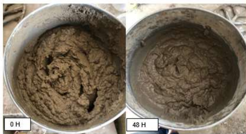
Figure 5 - Consistency of the 20% MC/10% EVA mortar at 0 h and 48 h.
